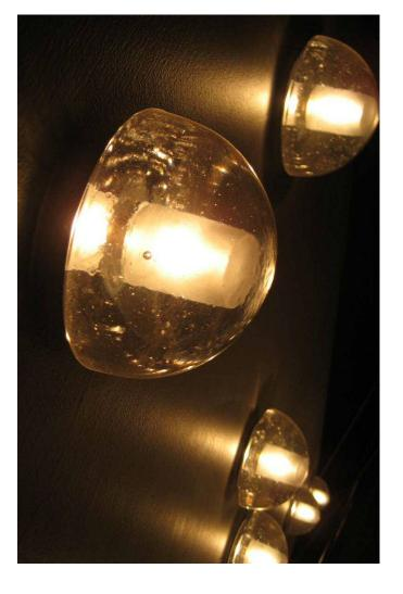
BOCCI 14 SERIES WALL SCONCE 4"H X 2"DEEP MADE OF CAST GLASS; FROSTED VOID HOUSES A 10 WATT HALOGEN OR XENON BULB UP TO 5 SCONCES MAY BE CONNECTED TO A SINGLE CLASS 2 TRANSFORMER INCLUDES MINI JUNCTION BOX ITEM NO.LI93
