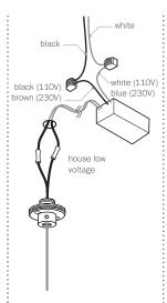
Connect the house wires to the coaxial cable using #16 butt splices (stagger the splices). Use raw butt splices and heat shrink to simplify the installation.
