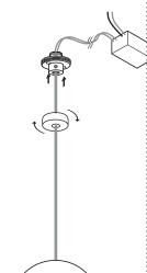
Affix mini-canopy to ceiling surface with fasteners provided. Twist the threaded canopy cover plate into place.
