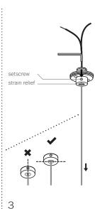
Determine the overall drop for the pendant fixture. Use the Allen key provided to loosen the setscrew in the canopy and gently feed the cable through the canopy until you have reached your desired drop length. Use Allen key to tighten the setscrew to hold the strain relief to secure the coaxial
