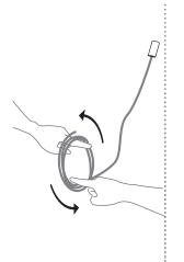
Very carefully uncoil the braided coaxial cable in a spool like manner. Insert your index fingers into opposite sides of the roll then rotate your fingers around each other to unroll the coaxial cable. Use patience: allow the cable to uncoil completely to avoid kinks.
